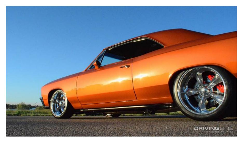
CPP Stage IV tubular A arms, QA1 coil overs and C5 spindles up front give the Chevy the maneuverability and handling qualities of a modern sports car, while the CPP Stage IV adjustable 4-link with Viking coil over shocks help keep the GM 12-bolt, limited-slip rearend with 3.55 gears and narrowed 3 <sup>1</sup>/<sub>4</sub>-inch Moser 31-spline axles floating effortlessly above the pavement and pushing the performance car to top speed.
