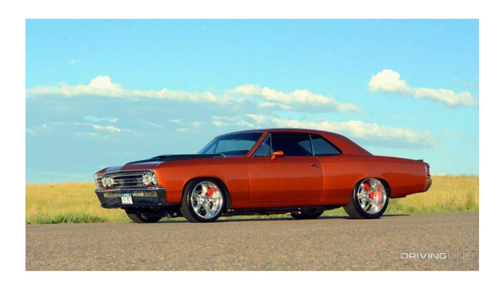
Planting the car to the pavement are 18x8" (front) and 20x12" (rear) American Racing Torq Thrust wheels with 4 ¼" and 4 ¾" backspacing, accordingly. Behind those you'll find 14" slotted and cross-drilled Baer brakes with 6-piston calipers on all four corners.
